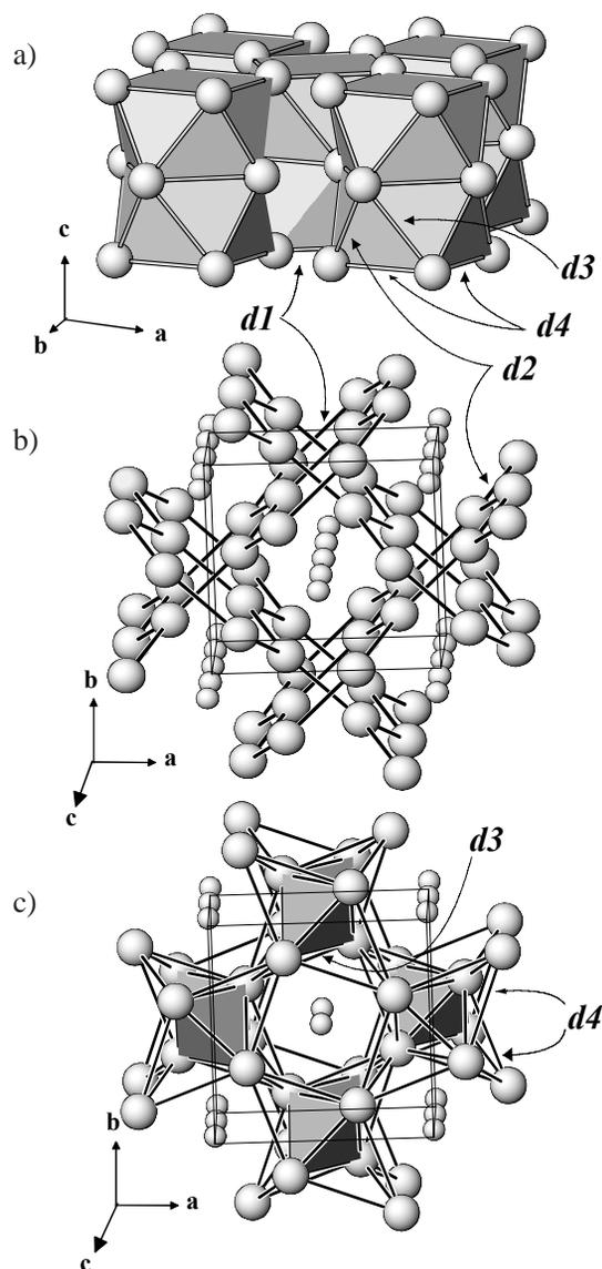
Fig. 1: The different representations of the  $\text{CuAl}_2$  structure type (small spheres:  $A$  atoms; large spheres:  $B$  atoms).
