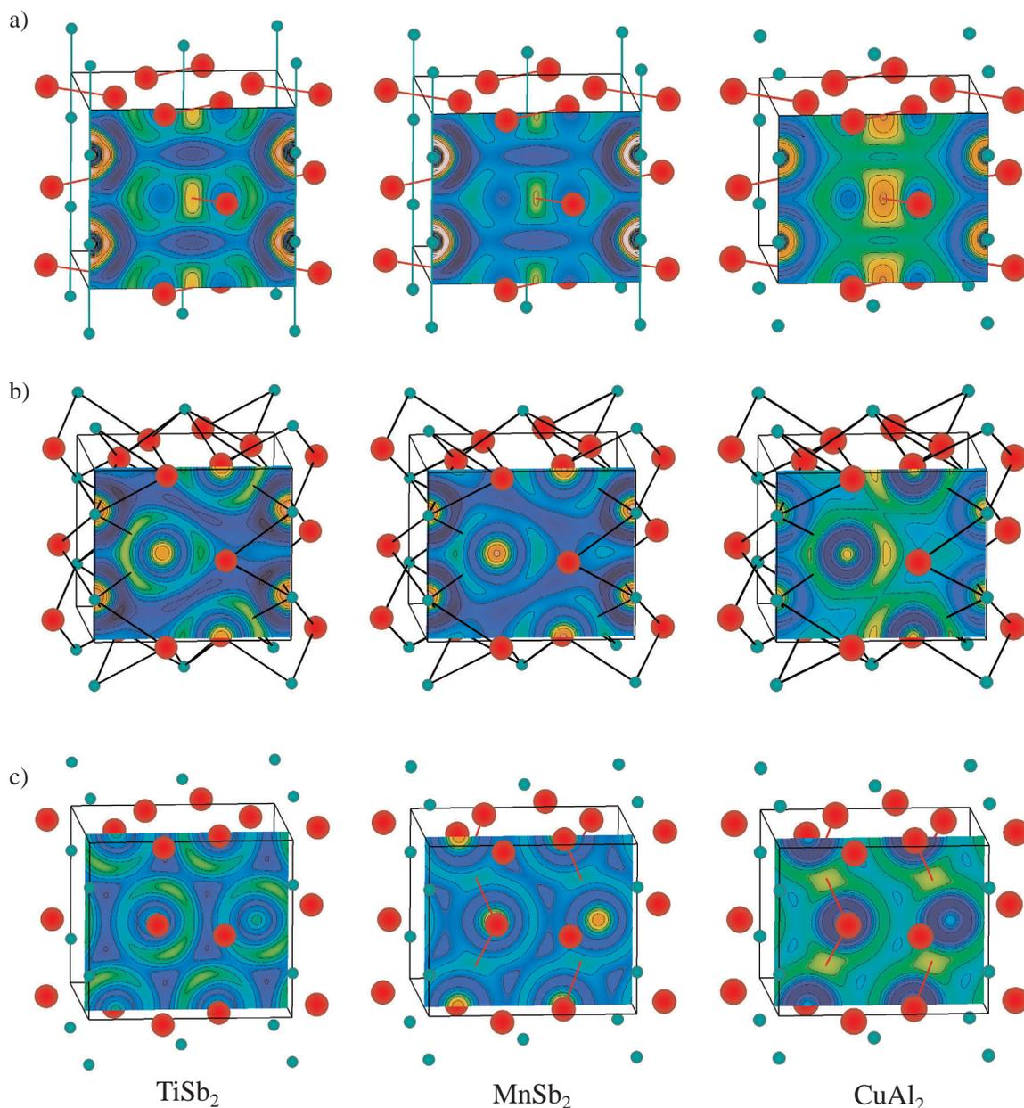
Fig. 2: ELF for representatives of the  $\text{CuAl}_2$  structure type. The ELF slices are crossing the middle of the distance  $d1$  and include the shortest A-A distance (a), the center of the three-center A-B-A bond (b), and the middle of the distance  $d2$  (c). A maximum in the ELF (yellowgreen/yellow/orange) is indicating covalent interaction (green: A atoms; red: B atoms).
