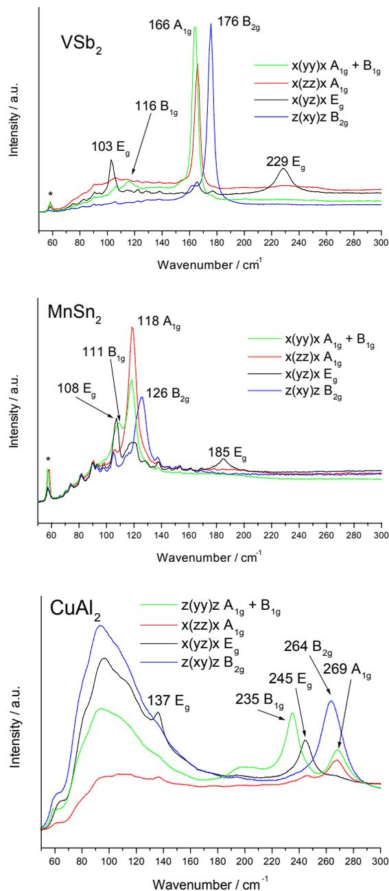
Fig. 3: Polarized Raman spectra of oriented single crystals of  $\text{VSb}_2$ ,  $\text{MnSn}_2$  and  $\text{CuAl}_2$ . In each polarized measurement only modes of a certain symmetry are allowed (\* grating ghosts).
